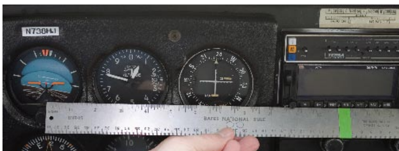
The Garmin GNS 250XL in this Cessna is well within the 11.8-inch acceptable viewing area, so upgrading to a WAAS-certified Garmin GNS 430/530W would require no annunciators.
