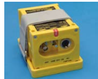
Martec Group's compact Kannad 406-AF compliant ELT pack
