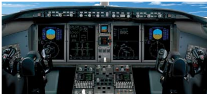
This Bombardier Challenger features the Rockwell Collins Pro Line 21, which is a true IFD.
