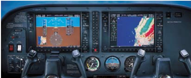
Although the Garmin G1000 in this Cessna Skyhawk panel has separate “boxes” behind the panel, it functions as a truly integrated flight deck.
