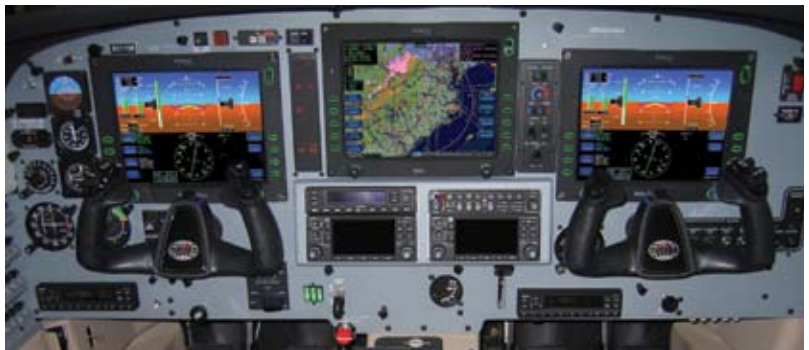
From the pilot's perspective, the Avidyne Entegra, such as the one in this Piper panel, functions as a true IFD.
