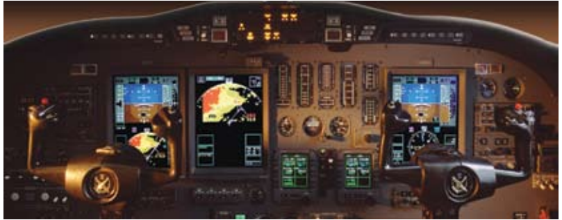
The Honeywell Primus Epic is a truly integrated IFD with all sensors, radios and others items in a central unit.
