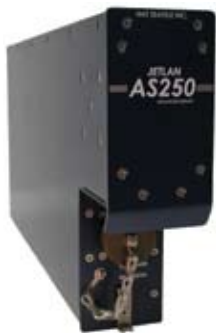
NAT Seattle's JetLAN AS250 advanced airborne computer
