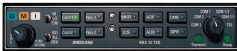
Honeywell's KMA 28, offers a complete set of controls for all the latest radios and passenger entertainment systems.
