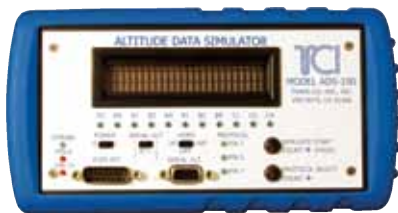
Trans-Cal Industries' ADS-100 altitude data simulator.
