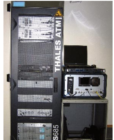
This data concentrator sends information to an aircraft controller’s console.
